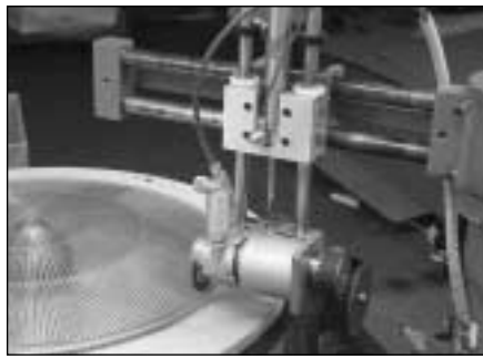
State-of-the-art compression machine ensures integrity of seal for hosedown luminaires
