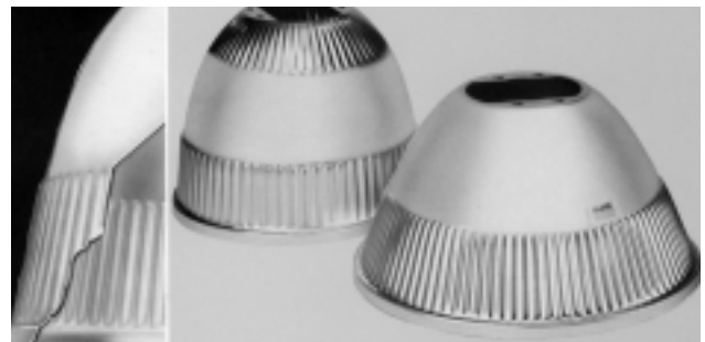
Vue-Trol Ribs function as a highly efficient diffuser to take the glare out of light. Patented ribs control brightness in the 60°-90° viewing zones and reduce glare up to 75% with no loss in efficiency.
